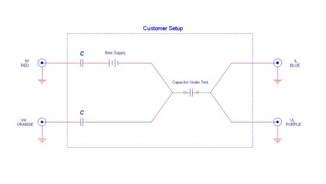
Measurements should be with the LCR Bias Voltage off. Allow the measurements to settle after the bias voltage is applied or changed.
